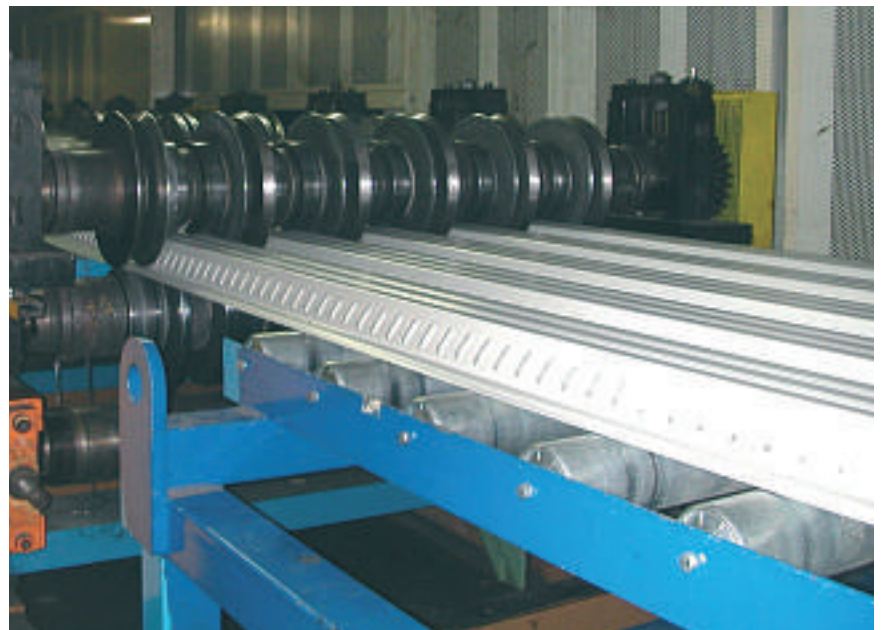
Fabrication of a composite floor deck
