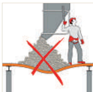
8. Ensure that there is no concrete accumulation
