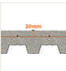
Fitting of reinforcements
