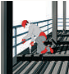
Fixing and stitching of the floor deck
